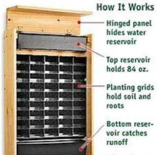
Living walls are vertically constructed gardens suitable for the interior of a building, which provide numerous environmental and health benefits. Living walls are relatively simple installations that can greatly enhance the quality of a space. This brochure provides a guide of how to construct your own indoor living wall so that you can start enjoying its benefits immediately.
